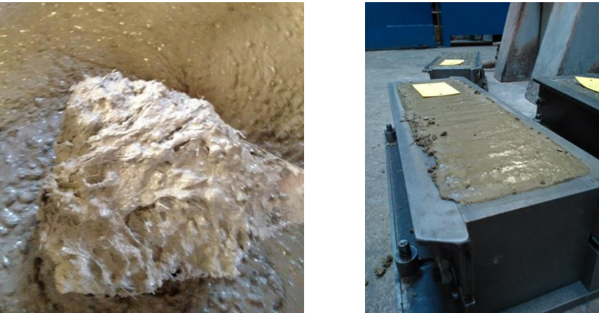
Fig. 9 UHPFRC in fresh state with thixotropic properties (left) and sampling during lab testing (right)
