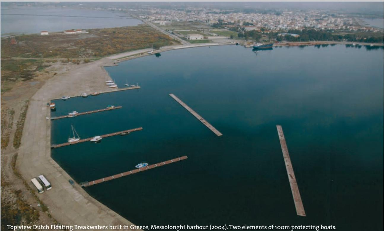
Top view Dutch Floating Breakwaters built in Greece, Messolonghi harbour (2004). Two elements of 100m protecting boats.
